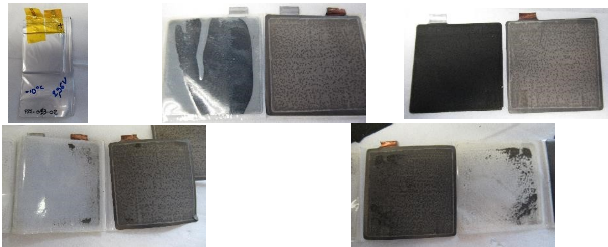
Figure 107 : Photos of the internal components of the STD02 cell (cycled at -10°C, 5 cycles, SOH = 57.57%) taken during the disassembly of the cell
