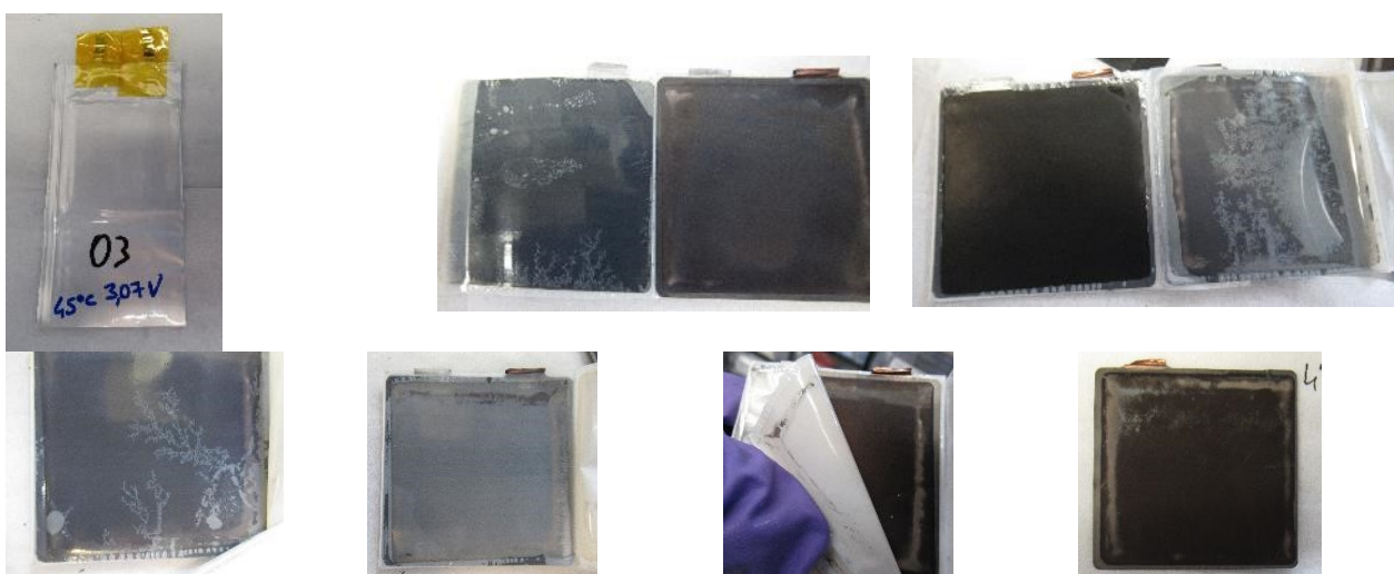
Figure 109 : Photos of the internal components of the STD03 cell (cycled at 45°C, 200 cycles, SOH = 85.81%) taken during the disassembly of the cell
